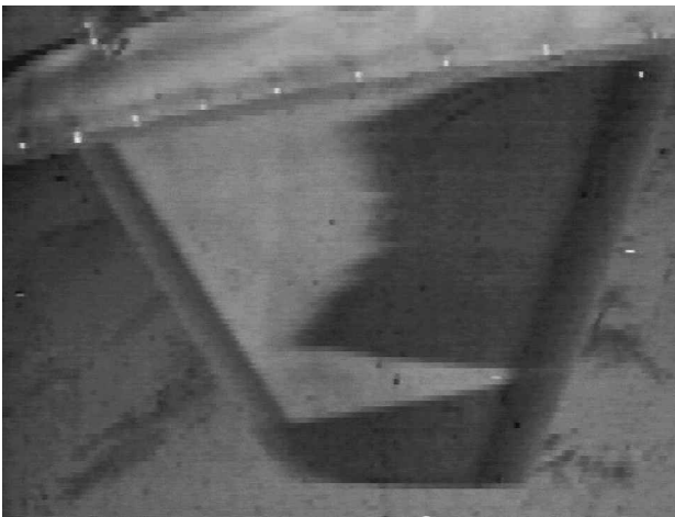
Fig. 11 Infrared image of test article during Flight 168: t = 10:02:11 (PDT), h_p = 39,500 ft, M_\infty = 1.59 .
